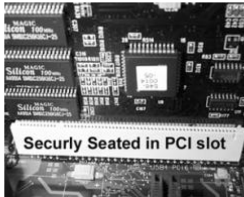
Figure 4-4 The expansion card above is seated properly in the PCI slot. Note that it is difficult to see the pins in the slot as well as the notch. The card is level in the slot.
