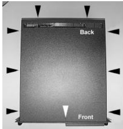
Figure 4-1 Location of the lid screws on Heavy Metal systems.
